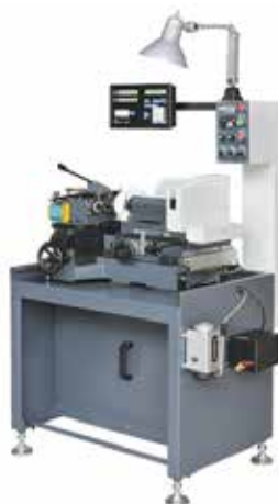
ROLLER TYPE EXTERNAL GRINDER H-18SP WORKPIECE DIA Ø1-25 MM GRINDING WHEEL 100 X 20T X 25.4 MM
