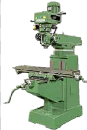
VERTICAL TURRET MILLING MACHINE 16-SERIES X / Y / Z TRAVEL : 850 (OPT 950) / 426 / 400 MM SPINDLE TAPER : R8 NT30 SPINDLE MOTOR : 3HP
