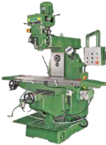
VERTICAL & HORIZONTAL MILLING X / Y / Z TRAVEL 1000 (OPT 800) / 400 / 470 MM SPINDLE TAPER NT40 SPINDLE MOTOR 5HP (OPT 7.5 HP)
